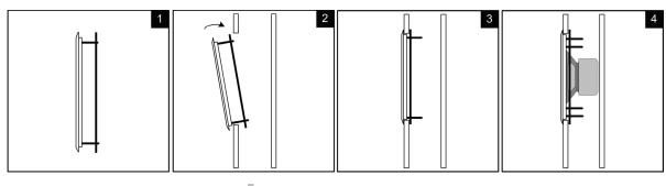
the speaker location on the wall. The PCB-LCRS brackets are available from the distributor or dealer where the speakers were purchased. When the brackets are used the holes are cut when the drywall is installed. The cable can be tied off on the bracket after securing the cable to a nearby joist.
