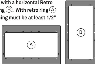
Once the speaker locations are established use the cardboard template (the outside of the inner cardboard rectangle) to mark the speaker cut-out. The dimensions for the cut-out are listed on the previous page. Using the proper tool, cut the appropriate sized hole in the wall. On drywall, clean cuts can be made with a drywall saw.
