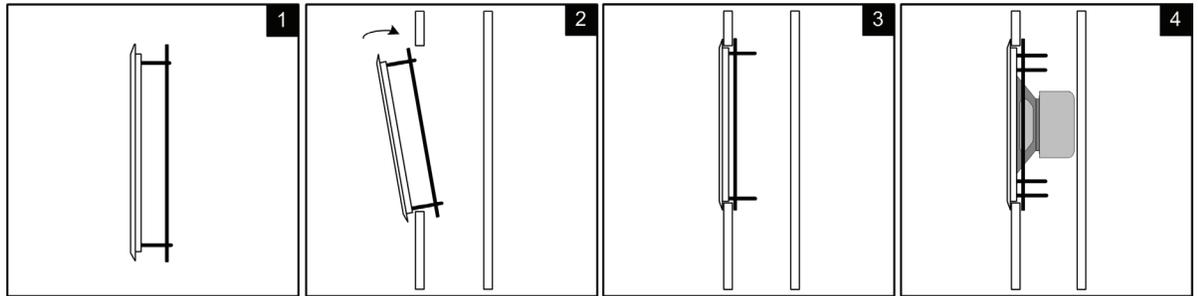
The AKF-5.25LCRS is shipped with a horizontal Retro Ring (A) and a vertical retro ring (B). With retro ring (A), the edge of the speaker opening must be at least 1/2" (13mm) away from a stud if the speaker is installed in the portrait orientation. Retro ring (B) is for mounting closer to the stud when in the portrait orientation.
