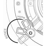
This speaker is optimized for off-axis listening through the use of a pivoting tweeter and a 15 degree baffle tilt. We recommend directing the woofer and tilting the tweeter toward the listening
